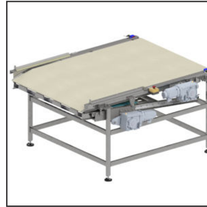
Feeder table for dough taking out from baskets and for operating with loading side setters
